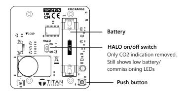
The sensors are supplied with a battery tab in place. Remove this before attempting to commission the device.
