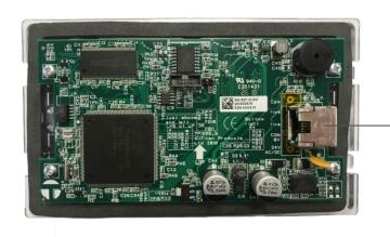
RJ45 connection to controller. RDU is powered from this connection reducing site wiring.
