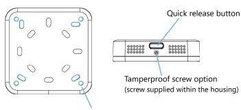
Recommended mounting holes for direct to wall (no back box)
