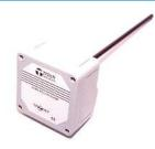
The Titan Products Wireless Duct Humidity & Temperature Sensor is designed to wirelessly monitor the air flow humidity and temperature levels in pipe work. This measurement is then transmitted over a Zigbee wireless network back to the Titan Products Co-ordinator.
