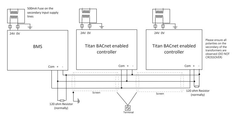
The above diagram shows a typical 3-wire daisy chain configuration. For all BACnet standard wiring variants please consult ASHRAE wiring standards.
