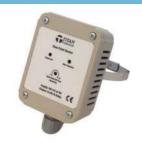
The TPDP Dew Point Sensor is designed for applications with chilled beams and other cooling coils to prevent the onset of condensation. There are two versions, the clamp-on (TPDP/CS) or flying lead (TPDP/FL).
