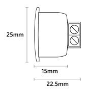
The TPFMTS is also available with a 2 wire, resistive flying lead assembly (TPFMTS/FL). The flying lead is 5m as standard however other lengths are available.
