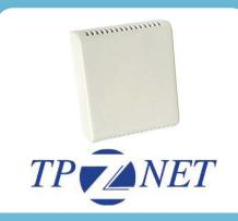
The Titan Products Wireless Room CO2 & Temperature Sensor is designed to wirelessly monitor the CO2 and temperature levels of a space and transmit the data over a Zigbee wireless network back to the Titan Products Co-ordinator. There is also an option to add a humidity sensing point to the sensor.
