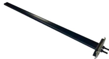
The Velocity Probes with multiple holes along the length are designed to measure the average velocity pressure across air ducts. The multi-point measurements offer an improved accuracy of measurement over the single point method.
