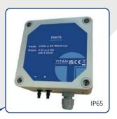
The TPAVT8 Air Velocity Transmitters are designed for applications in ventilation, fan speed control and air velocity control. The TPAVT8 employs a solid state temperature compensated differential pressure cell with microprocessor to provide superior linearity, measurement accuracy and sensitivity.
