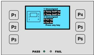
When a key is pressed to proceed then the following display appears to allow setting of fan speed and temperature.
