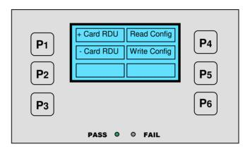
For security purpose the Read Config action from the connected controller into the FPT is protected from misuse. The following is displayed and requires confirmation of selection by an entry code 1,2,3,4 to proceed. Use the display instructions to enter the 1,2,3,4 then press **P3 OK** to proceed.
