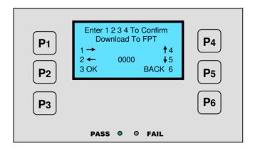
The FPT-601 now starts the read and Overwrite of the existing FPT Config from the connected controller. The Pass light at the bottom is continuously lit during the Download to FPT process.
