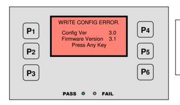
This display shows the config version in the FPT and Firmware version in the target control device. If these are incompatible then a new Write Config String will not be allowwed
