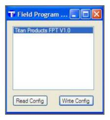
Once the "Read Config" is complete the FPT-601 config file is Uploaded in to the PC and the following Dialogue boxes appear: - "Config File uploaded" followed immediately by "Save Config File"
