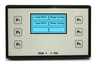
The FPT-601 Field Programming Tool is designed for commissioning, setup and configuration of the TITAN BACnet enabled controllers with firmware of V3 onwards
