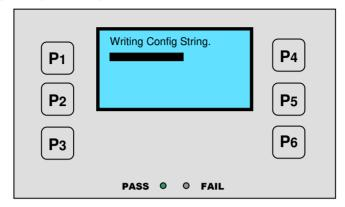
When the Write Config String is complete the following is displayed with a Green backlight. The Alphanumeric reference will be different dependant on the config reference number and the control device being read from.
