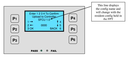
Once confirmation of the Write Config is selected by pressing P3 (OK) the display shows a dynamic bar during the process of Uploading the config file.
