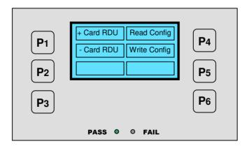
Select the type of RDU by pressing P1 (Card RDU) or P2 (Non Card RDU) once the selection is made then the one of the following is displayed with a request to confirm the selection by pressing P3 Yes or P6 No
