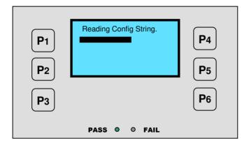
When the Read Config String is complete the following is displayed with Green backlight. The Alphanumeric reference will be different dependant on the config reference number and the control device being read from.
