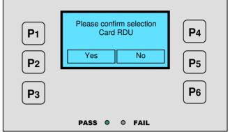
When Yes (P3) is selected and dependant on the RDU type one of the following will be displayed providing information on the function keys to be used.
