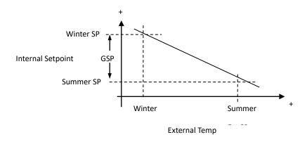
The following settings need to be entered if externally compensated adjustment is used for the GSP
