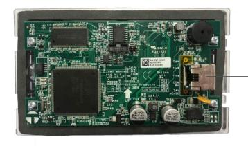
RJ45 connection to controller. RDU is powered from this connection reducing site wiring.
