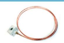
The duct averaging temperature sensor is designed to measure the average temperature across a duct to eliminate the effects of air stratification.
